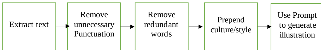
Figure 10: Prompt Processing pipeline
