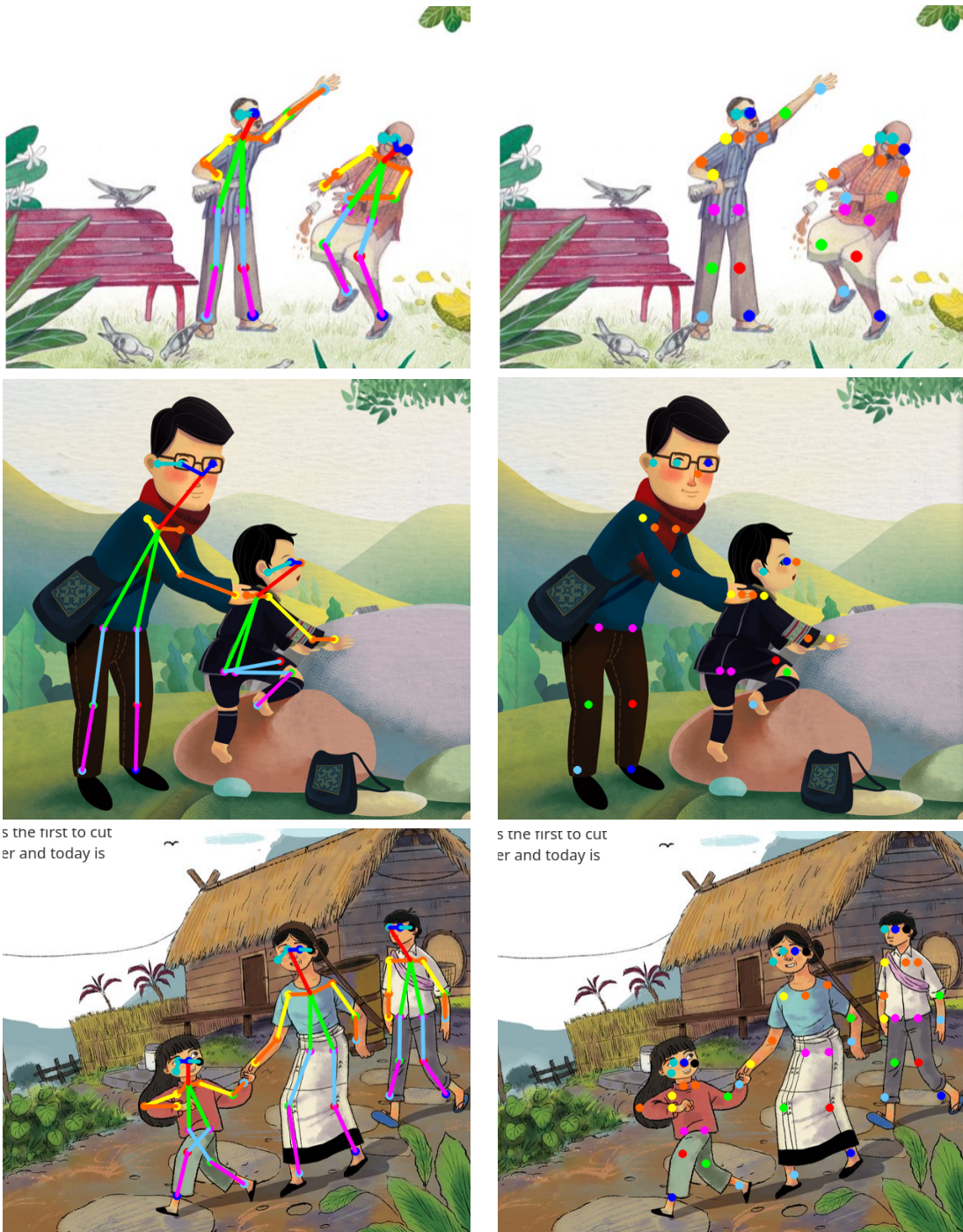
Figure 3.11 - Open pose estimation technique, which detects the body shaping of a human instance by detecting its joints [38]
